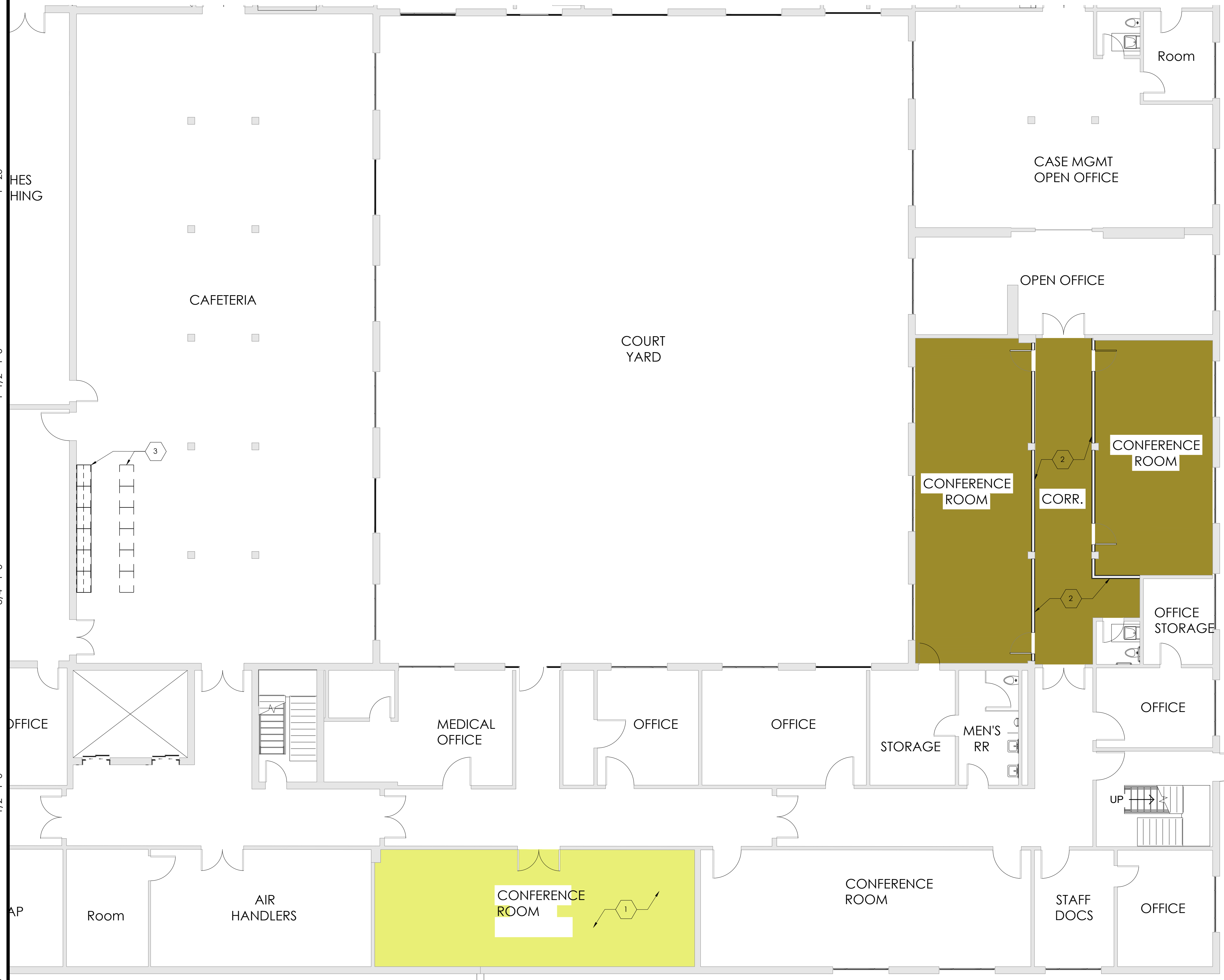
1 LOWER LEVEL DEMOLITION PLAN A2.0 3/32" = 1'-0"
